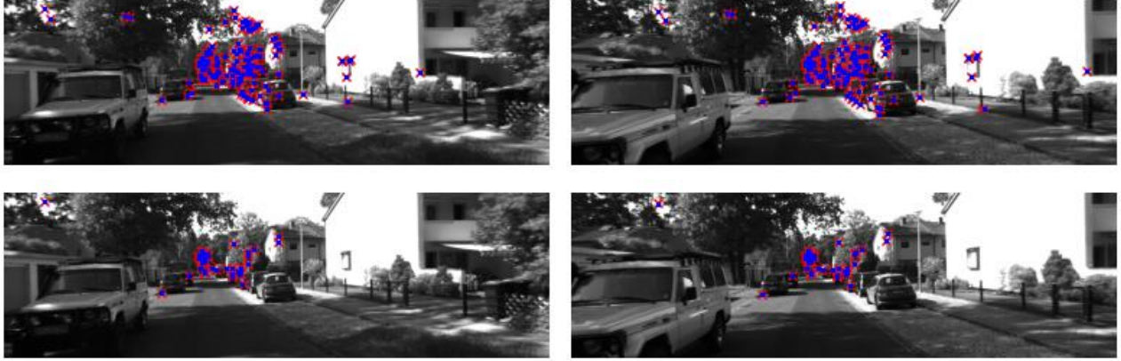
Fig. 5. Qualitative examples from two frames of the KITTI dataset (on sequence 0022 from 09/26/2011) [7]. In the images, the 2D detected points for inliers are shown in blue , whereas the corresponding reprojected 3D points are shown in red . The two frames on the top used the visual-only optimization method, while the two frames on the bottom used visual-inertial optimization. The visual-inertial optimization results show significantly fewer inliers.
