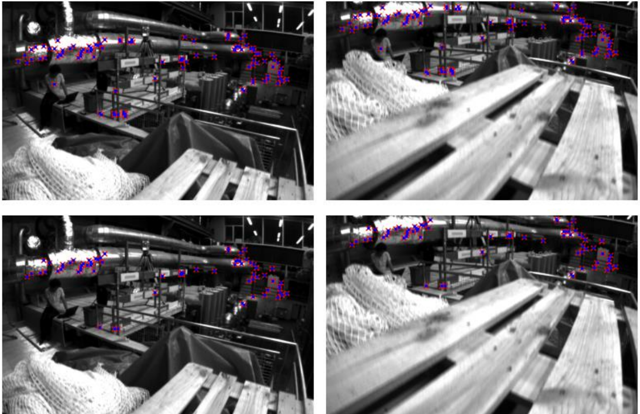
Fig. 6. Qualitative examples from two frames of EuRoC MAV (on sequence Machine Hall 01) [1]. In the images, the 2D detected points for inliers are shown in blue , whereas the corresponding reprojected 3D points are shown in red . The two frames on the top used the visual-only optimization method, while the two frames on the bottom used visual-inertial optimization. The visual-inertial optimization results show fewer inliers.
