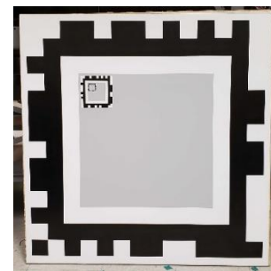
nested multi-scale fiducial marker
