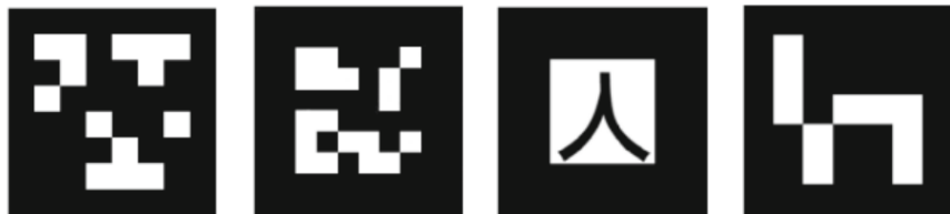
The examples of various fiducial markers: AprilTag, ARTag, ARToolKit, and ArUco, from left to right
